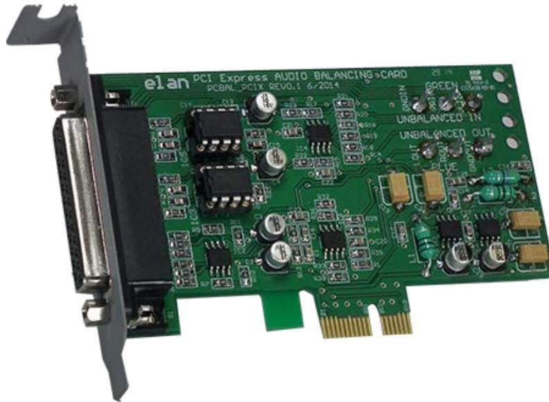
The PCBAL-PCIX is a plug in board for personal computers designed as a quality stereo interface between balanced +4 dBu standard broadcast line level systems and unbalanced computer sound cards.
