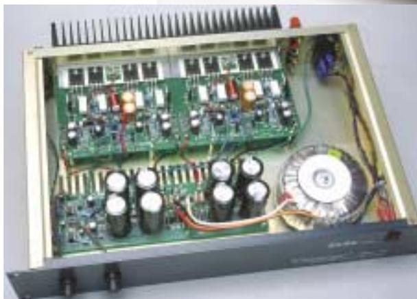
stages, each with their own current sources. The output stage employs rugged 40MHz complementary bipolar transistors, considered by Elan Audio (and us!) to produce better quality sound than power Mosfets.
